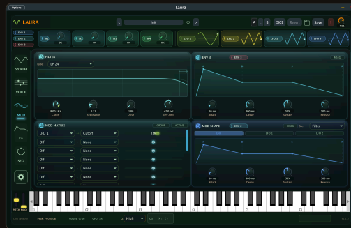
THE MOD PANEL. THE FILTER, THE THIRD ENVELOPE (ENV 3), A SIXTEEN-SLOT MOD MATRIX, AND THE MSEG MOD-SHAPE EDITOR. FOUR LFOs AND THREE ENVELOPES ROUTE FROM THE TOP STRIP.
