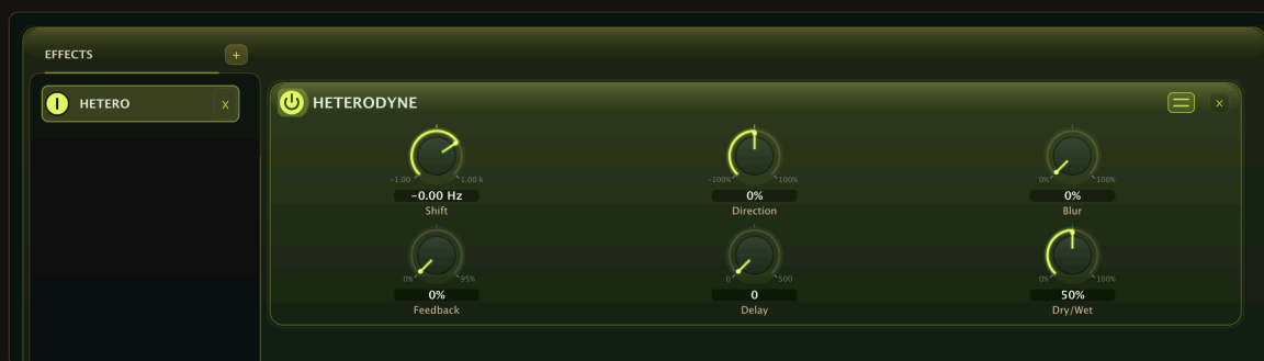
THE HETERO MODULE. HETERODYNE FREQUENCY SHIFTING.
