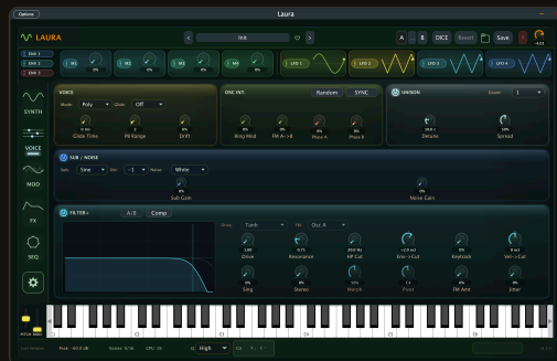
THE VOICE PANEL: VOICE MODE AND GLIDE, OSCILLATOR INTERACTION, UNISON, SUB/NOISE, AND THE FILTER.
