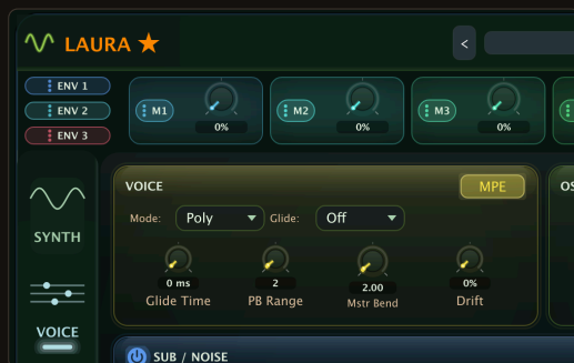
THE VOICE PANEL. THE MPE BUTTON SWITCHES PER-NOTE EXPRESSION ON; PB RANGE IS THE PER-NOTE BEND RANGE, MSTR BEND THE MASTER WHEEL RANGE.
